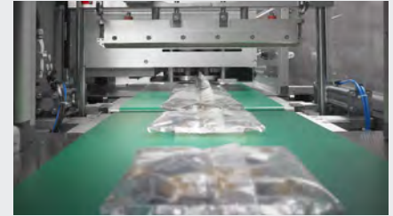
Guillotine-type or box-motion cross sealing system
